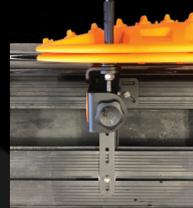
17. Check that the brackets are aligned at 90° to the platform planks, then tighten the nyloc nuts on the channel bolts sufficiently to ensure that both bracket assemblies are securely fastened to the platform and cannot move.
