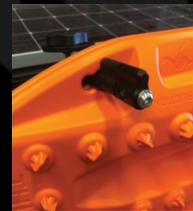
16. Place 2 **MAXTRAX** onto the mounting pins and turn the knuckles 90° to hold the **MAXTRAX** in place.
