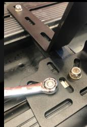
15. Repeat **Steps 10 to 14** for the second bracket assembly, except **DO NOT** fully tighten the Nyloc nuts.
