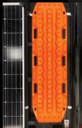
10. Slide 4 of the channel/slot on the outer side of the platform. Locate 2 of them (approximately 50mm apart) at the position from **Step 9**, and the other 2 (approximately 50mm apart) approximately 890mm (towards the rear of the vehicle) from the first 2 channel bolts.
