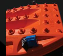
21. Install a padlock through at least one of the mounting pins to protect your **MAXTRAX** from theft.
