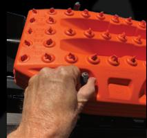
20. Install the **MAXTRAX** onto the mounting pins and turn the knuckles to secure them.
